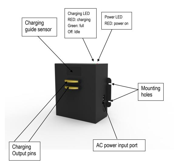
Installation guide: Please put this charging dock against a flat wall, make sure the front of charging dock is empty enough (> 2.0 meters @  $120^{\circ}$ ), without any obstacle in this area.
